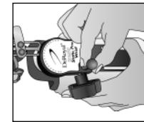
engagement knob (1) outward and at the same time pivot the position adjustment knob (2) back toward the elbow. The handcuff should move freely. **Note:** The adjustment knob should be positioned below the wrist in order for the device to achieve full extension.
