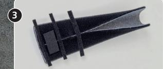
Start to create the circular shape by putting the material side-by-side and securing it with the hook strips. Try to keep the same distance between the strips, approx. 10–12 mm. Apply the NRX® Heat Tape pieces in between the strips. Make sure that they are not wider than the distance between the strips as this will make it difficult to remove the strips once laminated.
