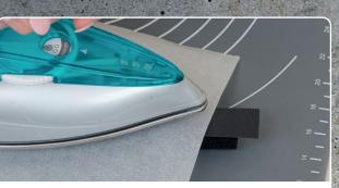
Cut another piece of NRX® Heat Tape that covers the full length of the sleeve plus 1 cm on each side. Position it so it covers the heat tape pieces. Repeat the lamination with the iron and make sure to cover the tape with a baking paper or Teflon sheet. Press for 10–15 seconds then let cool.
