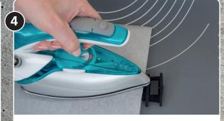
Position the tube on a heat resistant surface. Cover the material with a baking paper or Teflon sheet. Set the iron on medium heat (two dots) and press the NRX® Heat Tape for 10–15 seconds. Check that the edges has bonded. If not, repeat the process. Then let the material cool for 1–2 minutes before the second lamination.
