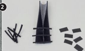
Cut 8–10 thin strips of NRX® hook that will be used to hold the construction together during the lamination. Then cut small pieces 8–10 mm in length of NRX® Heat Tape that should fit in between the hook strips.
