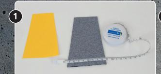
Take the distal and proximal circumference of the finger and make a symmetrical paper pattern of the finger shape. Make the length of the pattern twice the length of the finger to have enough material to adjust the length of the sleeve afterwards. Choose the appropriate material for your application and cut it to the pattern.
