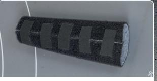
Remove the strips carefully. The heat tape must be completely cool. The tube is now held in place with the heat tape pieces.
