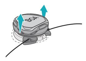
a. Insert flat-head screwdriver into the tab with an arrow indicator. b. Use tool to pry reel upward until cartridge pops out of bayonet.
