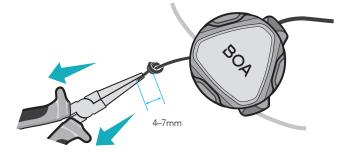
b) Determine lace length needed. Leave a maximum of 15cm of lace capacity per lace port.
