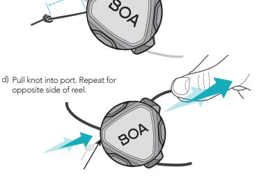
Note: Knot and tail should not be visible when the lace is seated properly.
