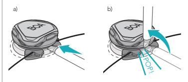
Note: Tab is located on top of mounting plate between the lace ports.
